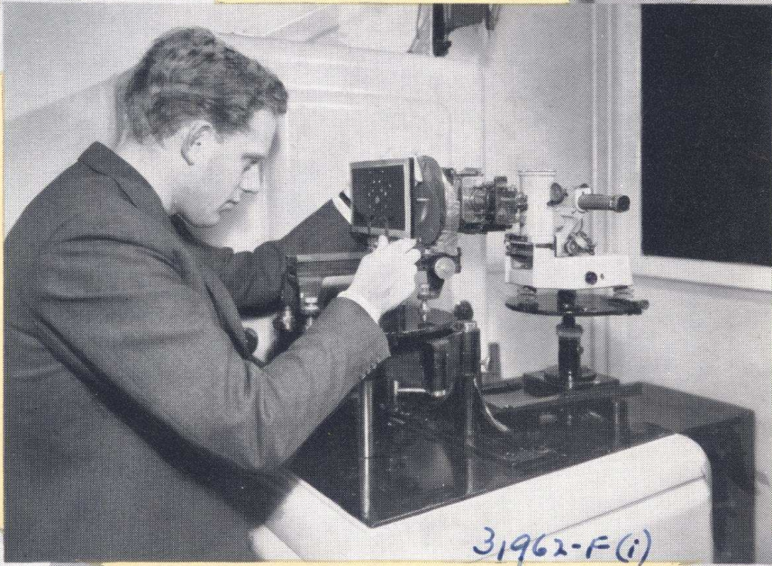
Apparatus for determining hardness at elevated temperatures in vacuo
