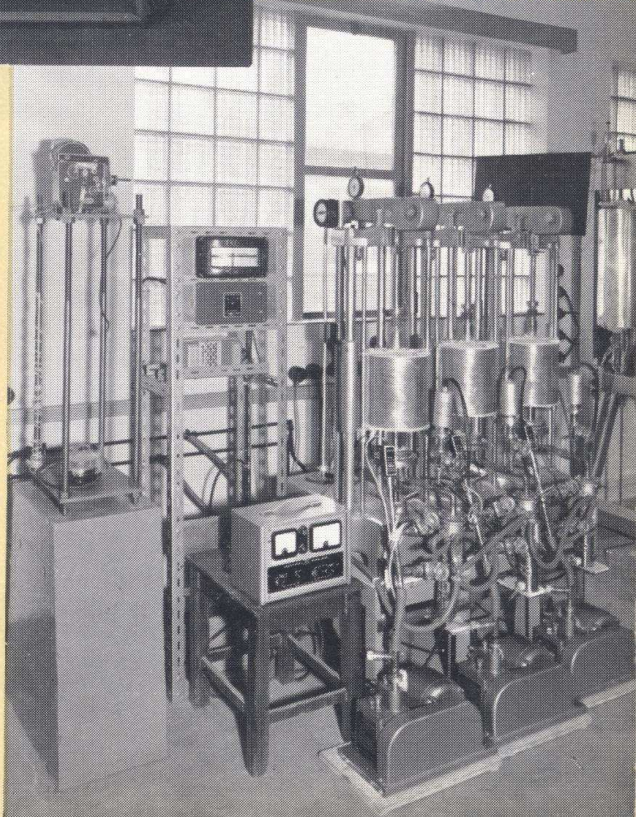
Creep testing in vacuo with continuous photo- graphic recording 31962-M.
