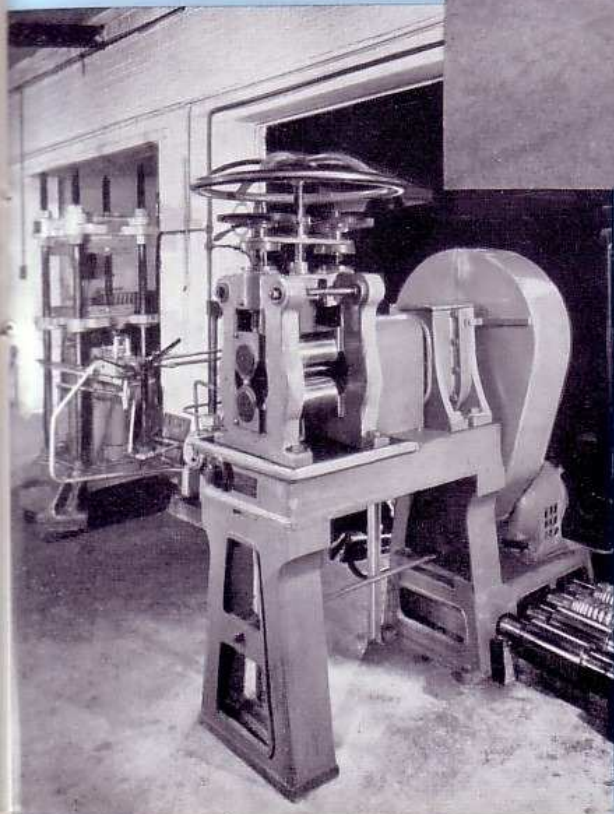
BELOW Rolling Mill
