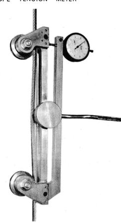
A simple method of measuring the tension in ropes has for some time been a requirement in designing yacht rigging. F.R.I. has designed and built prototype tension meters on behalf of Norseman Ropes and these may have a wider range of application, for example, in tie ropes for wireless aerials and transmitters and colliery winding gear. Both electrically recording and dial reading instruments are available. The latter is illustrated.
