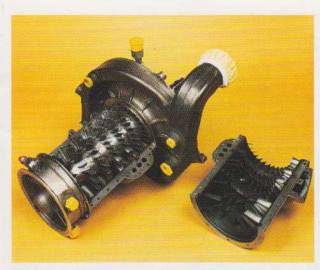
Failed helicopter gas turbine compressor module.
