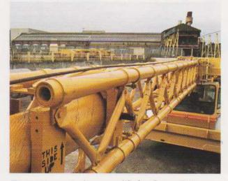
Prototype composite crane jib for Grove Coles.
